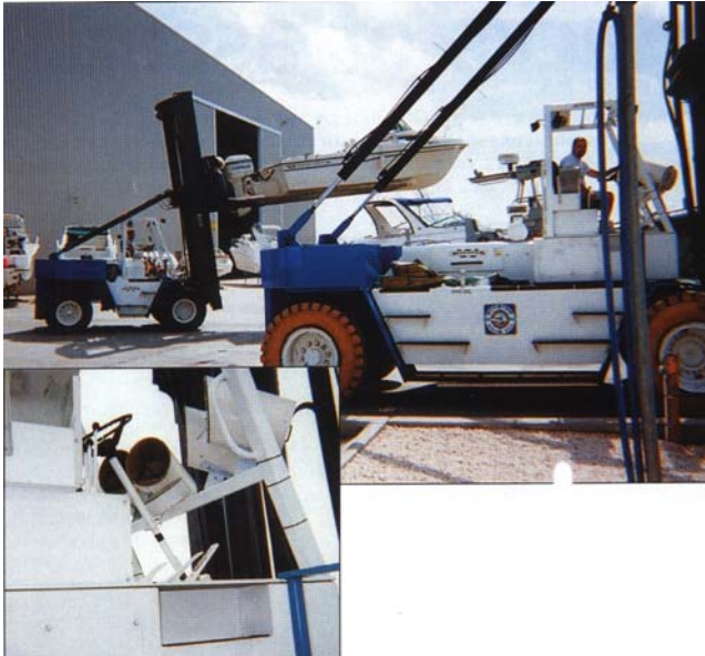
The 30,000 lb. Forklift has CCTV cameras with monitors (inset).
