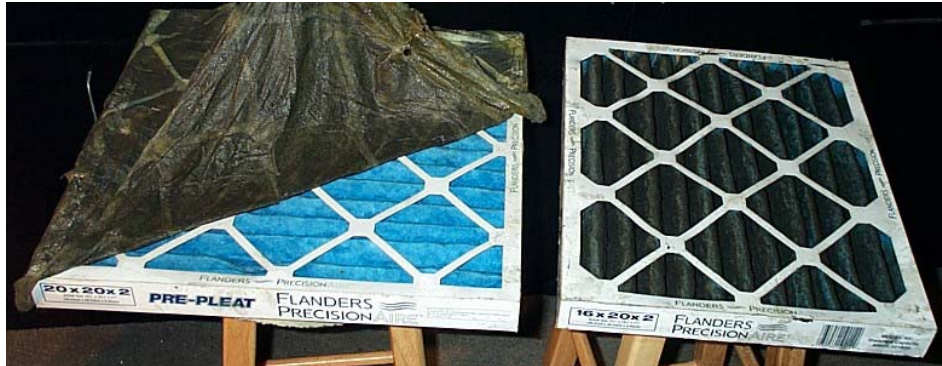
PS prefilter capturing oil mist
